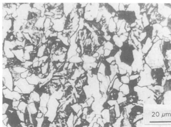
Figure 2 A typical representative microstructure of the investigated materials showing primarily a mixture of equiaxed ferrite and pearlite along with some acicular ferrite.
